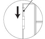
2. With hinge pins installed, open the left panel. Place the right shutter panel into the window opening and slide into position. Once the panel is aligned with the frame hinges, insert hinge pins into hinges to secure the panel.
