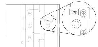
▲ To ensure panels are installed correctly: Identify the top and bottom of the panel by locating the top label on the top hinge.
