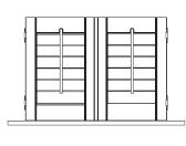
3. If you have bi-fold panels, after attaching the far left and/or far right panels to the frame in the previous steps (1 & 2), you will need to join the hinges of the panels labeled P1 and P2 and insert hinge pins. Repeat for panels labeled P3 and P4 if you have these. Proper order of panels from left to right is P1, P2, P3, and P4.
