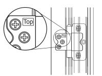
To ensure panels are installed correctly: Identify the top and bottom of the panel by locating the top label on the top hinge.
